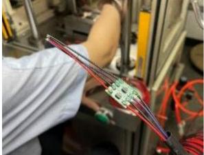
In addition to general over-molding MEGA also offers **low-pressure over-molding**. Lowpressure over-molding normally applies to the cable **with a PCB or IC** embedded and it helps to prevent PCB and IC damaged during the molding process.
