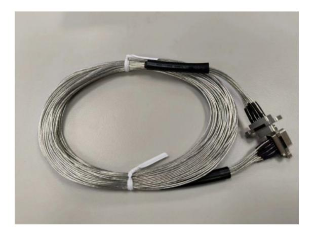
Teflon wire can be used in wide temperature environments (-50~250°C,) which can be required in extreme environments, such as steel processing equipment. Shown left is a harness to be used on oil drilling equipment, where it is not possible to use ordinary PVC or Silicone wire. Wire can be tinned or silver plated for stable signal transmission.
