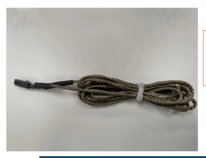
Specialized tinned copper wire twisted with nylon, also basalt fiber jacket for **leak detection** of server **cooling** liquid. This solution fulfills a requirement by performing in the harsh environment. MEGA has an expert engineering team for special wire/cable development.
