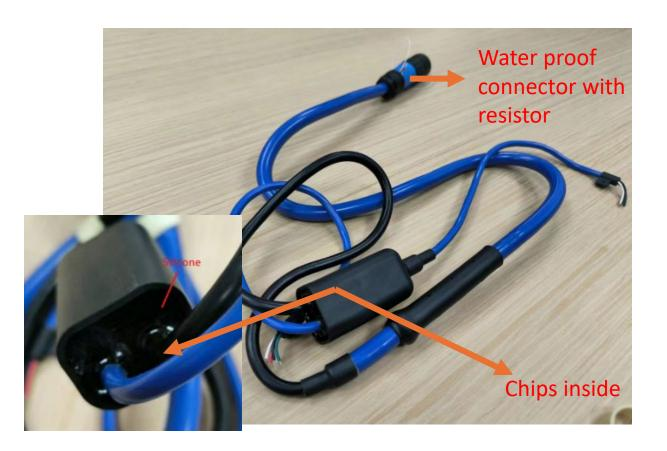
The key for making marine interconnecting cables is waterproof or watertight over molds.
