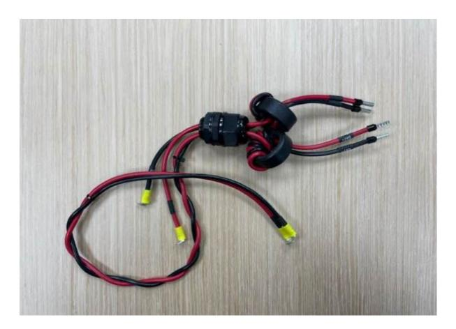
This is a unique product, requiring the winding of cable through the ferrites to be done manually and evenly **to reduce the impact from EMI.**
